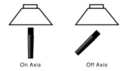
⑥ The serial number of the microphone placement. The smaller number is close to the center cap and the larger number is close to the cone edge.
