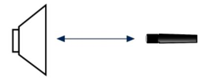
The on/off axis of the microphone placement.
