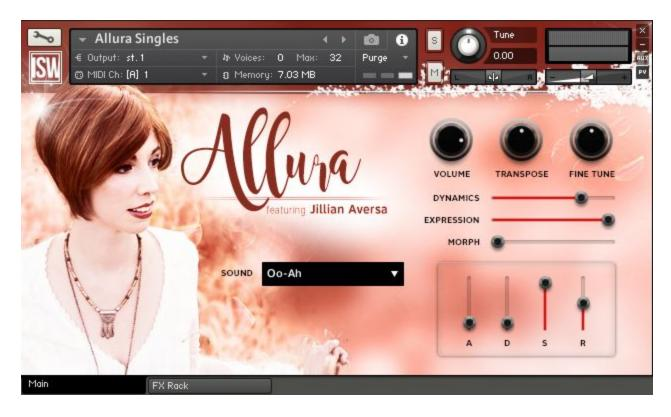
Use the **Sound** dropdown to select vowels or atmospheres, and the volume envelope (or **ADSR**) to sculpt it to your liking. With "Oo-Ah" selected, the **Morph** slider morphs between the two vowels. When an atmosphere is selected it serves to adjust filter resonance.
