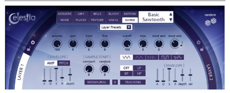
**Celestia** has a dual-layer architecture: two individual sound sources can be loaded at once, each with different volume, panning, tuning, filters, envelopes, etc. **All controls pictured above** are unique to each individual layer.
