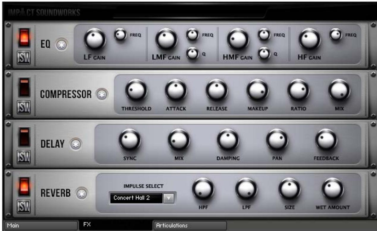
Our easy-to-use FX rack features an analog-modeled parametric EQ & compressor, delay line, and convolution reverb.
